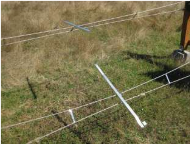
PV Hanger has a series of indents to capture cable
