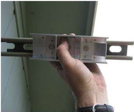
TCS Gable Mount Pivot Joint for R1 and R2 (New Design)
